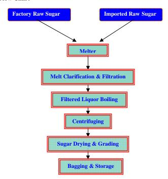
The detailed process of manufacturing sugar from raw sugar is described below.
