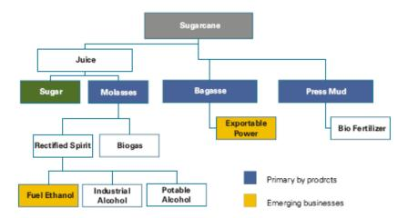
Fuel ethanol and surplus power production through cogeneration provide the two key by-products' related opportunities. Bagasse based cogeneration for exportable power is an emerging trend in the sugar industry. Bagasse generated by a sugar mill enables the mill to export power after meeting its captive power and steam requirements.
